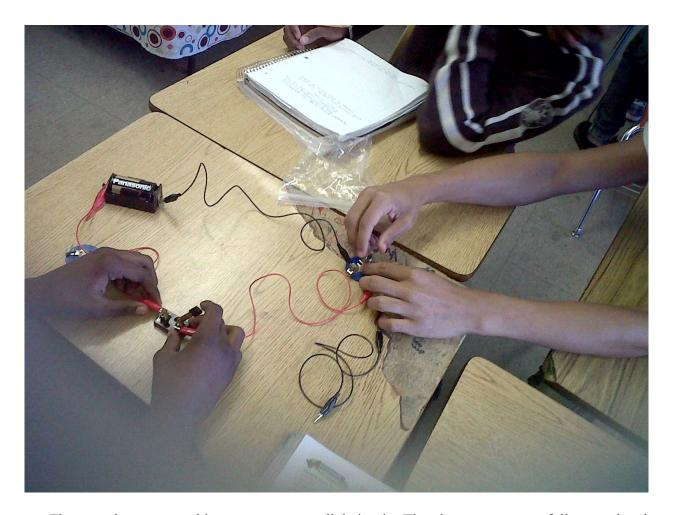
These students are working to create a parallel circuit. They have not successfully completed the circuit. When the switch is closed both bulbs light up, however when the circuit is open both bulbs turn off. A complete parallel circuit would allow one bulb to stay on when the switch is open.
